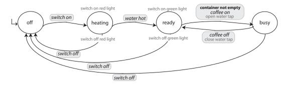
Figure 1. A graphical depiction of the state machine for a coffee maker
