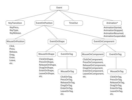
Figure 13. Classes of transitions available in SwingStates
