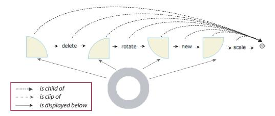
Figure 6. Relations between shapes in a control menu
