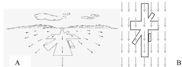
Fig. 5. The optical flow field available to someone onboard an aircraft when looking ahead (A) and downward (B). Fig. 5A reproduced from J. Gibson [9], Fig. 7.4 p. 124.
