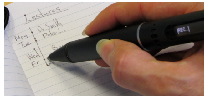
Figure 1. Drawing knotty gestures over handwritten notes about a series of lectures. Here, knotty gestures (dots on lines & characters) activate audio recordings and link them with the notes for future reuse.
