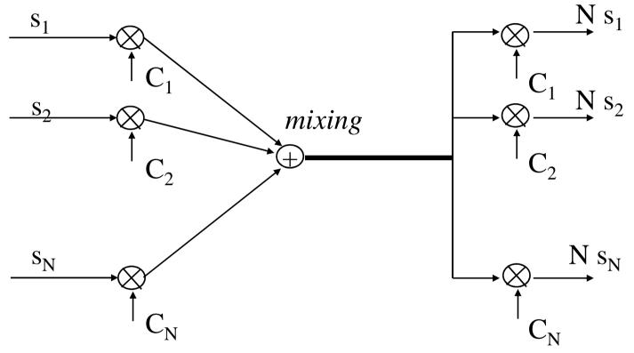
At the receiver: I can extract the k-th signal by simply multiplying by  $C_k$
