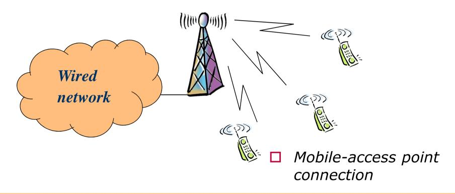
Cellular coverage: The territory coverage is obtained by Base Stations—BS (or Access Points) that provide radio access to Mobile Stations—MS within a service area called CELL
