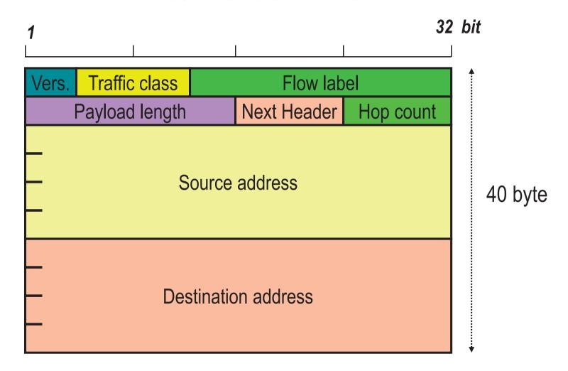
■ The Base Header length is <u>FIXED</u> (<u>40 bytes</u>)
