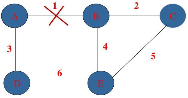
Ink 1 failure is detected by nodes A and B which send an LS update packet on *links* 3, 2 and 4 node A: From A, To B, Link 1, Cost=inf, Number=2 node B: From B, To A, link 1, Cost= inf, Number=2
