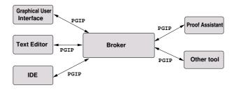
Fig. 2. PG Kit System Architecture
