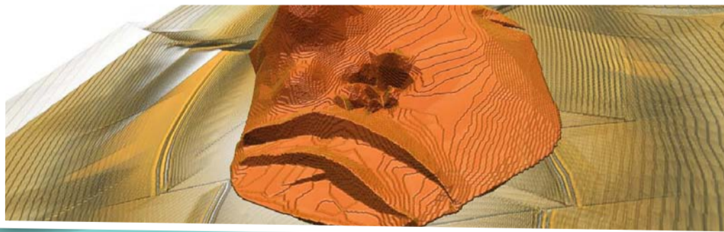
A synthetic velocity model of an oil and gas reservoir under a salt body
