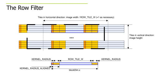
Figure 10: Layout of the thread block grid for the row filtering pass.
