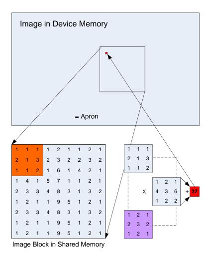
Figure 3: A naïve convolution algorithm. A block of pixels from the image is loaded into an array in shared memory. To process and compute an output pixel (red), a region of the input image (orange) is multiplied element-wise with the filter kernel (purple) and then the results are summed. The resulting output pixel is then written back into the image.
