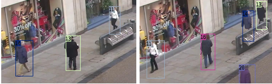
Fig. 7. Consistent people crossing over a span of 134 frames. The above images are cropped to show the crossing.
