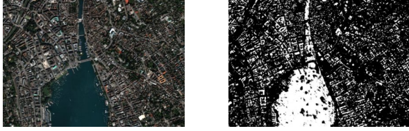
Fig. 1: A state-of-the-art CNN trained on a different dataset misclassifies most of Lake Zurich as a building.
