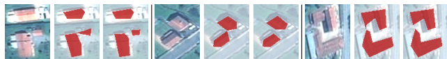
Fig. 7: Examples of color inputs (left) and approximation without (center) and with (right) topological constraints.
