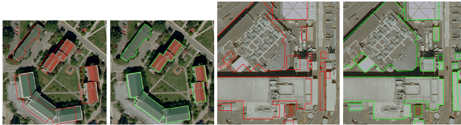
Fig. 1. Examples of multimodal image alignment. We align aerial images with cadastral images. For each example: Left: original image with OpenStreetMap (OSM) map (in red), right: after our realignment (result in green).
