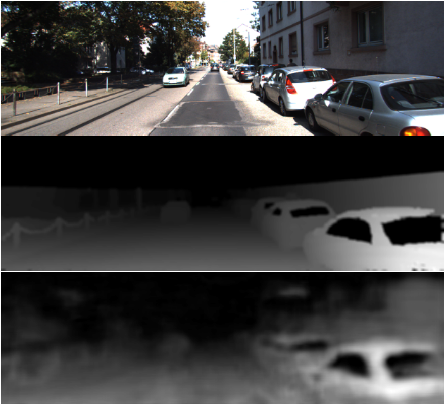
Fig. 2. Stereovision test. Top: right image; middle: ground truth depth map for right image; down: predicted depth map.
