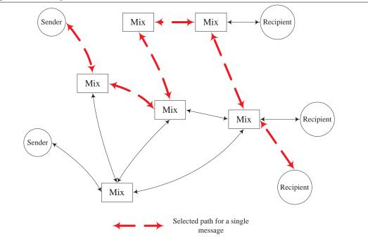
In general there are two possibilities of chaining Mixes together. In a *Mix network* the user can select an individual path through the network for each message. This is illustrated in Figure 2. Every Mix can send messages to all other Mixes (the arrows in Figure 2 show some message transmissions). The thick arrows highlight the path, which one sender has selected for his message.
