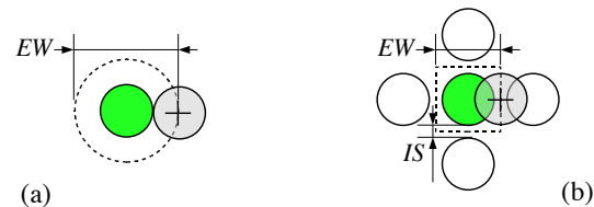
Figure 3. (a) Isolated target: potential effective width EW = W + SPOTWIDTH . (b) Small interspace between targets IS \leq SPOTWIDTH : potential effective width is EW = W + IS .
