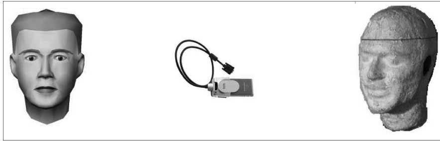
Fig. 7. The technical setup: the physical model of a human head used as a 3D projection surface, to the right; the laser projector in the middle; and a snapshot of the 3D talking head to the left.
