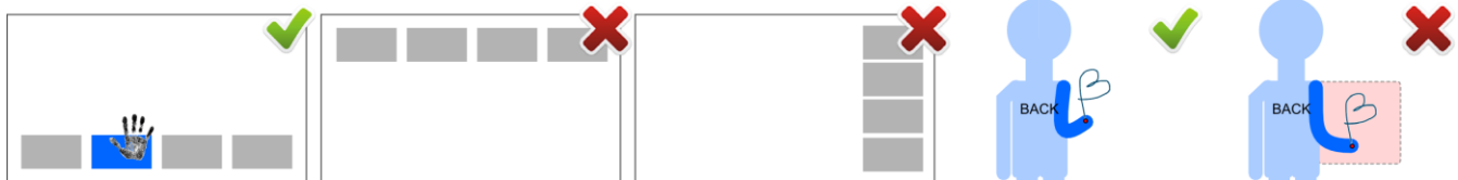
Figure 9. Design implications of consumed endurance. Left, menu items should be located in the bottom of the UI. Right, for some applications, such as free gesturing, designers may consider relative input which is possible anywhere in the interaction plane instead of a fixed location.
