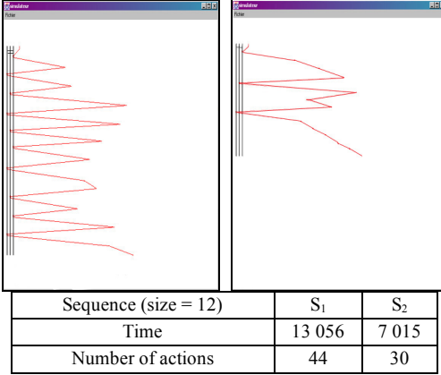
Figure 5: OMD and palette complexity for S_1 (left) & S_2 (right) Action complexity is computed as the number of nodes and the number of arcs in the path P . When a pre-condition is true, the corresponding arc and end node are not counted. Time complexity is computed by summing the time taken by each arc and node in P . The time taken by an arc is the sum of the time taken to choose that arc at the parent node and the time taken by the pointing action. The former is estimated by Hick's law [10]: k \log_2(1+n) for n arcs; the latter is estimated by Fitts' law [7]: a + b \log_2(1+D/W) for a target of size W at distance D . The time taken by a node is the constant time that labels the node. When the pre-condition of an arc is true, the time of the arc and its end node are ignored.
