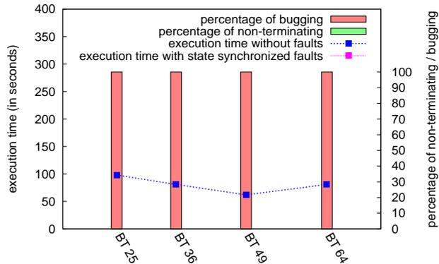
Figure 11: Impact of synchronized faults depending on MPI state
