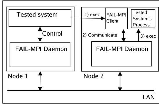
Figure 3: FAIL-MPI integration scheme
