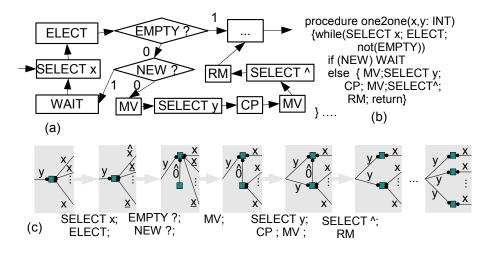
Figure 2. A graph-machine program (a) FSA (b) code (c) development.
