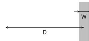
$$TM = a + b.ID \quad \text{où} \quad ID = id\left(\frac{D}{W}\right)$$
