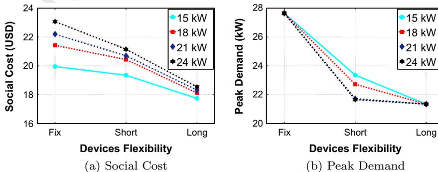
Fig. 8. SA-DSM results with 20 identical houses and a varying tariff threshold ( $\pi_{TT}$ ) of the pricing function.
