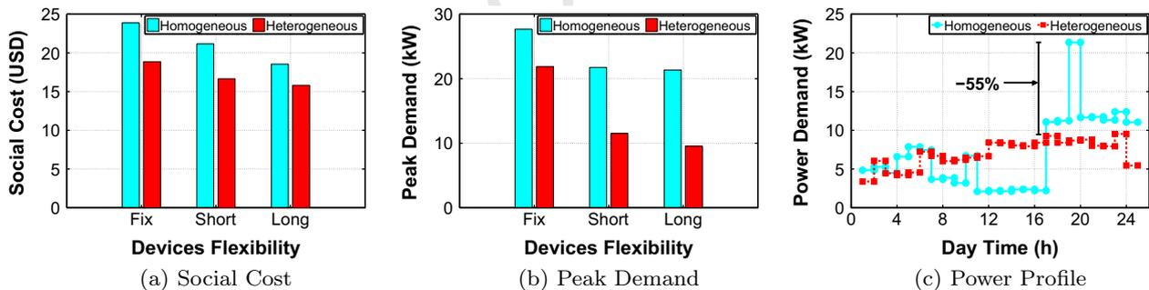
Fig. 7. SA-DSM results with 20 homogeneous and heterogeneous houses preferences.
