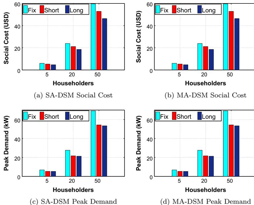
Fig. 5. SA-DSM versus MA-DSM system results considering homogeneous houses and a linear increasing cost function with minimum slope.
