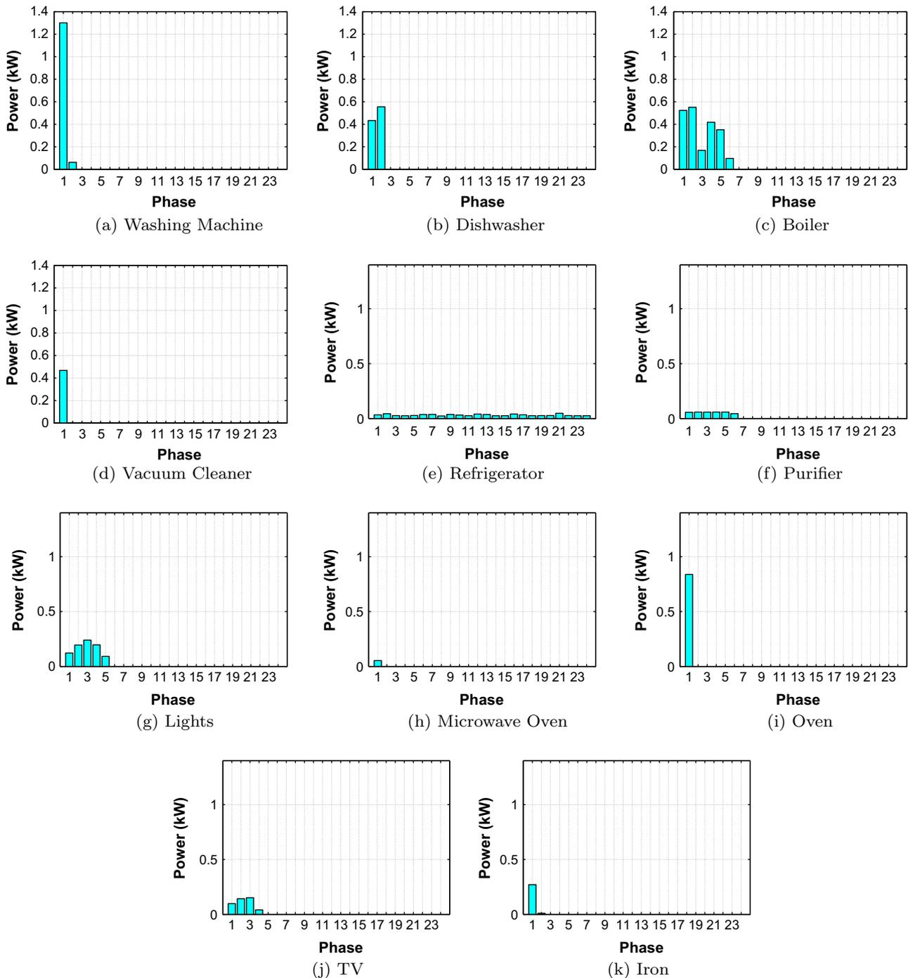
Fig. 4. Load profiles of the appliances considered in our tests.
