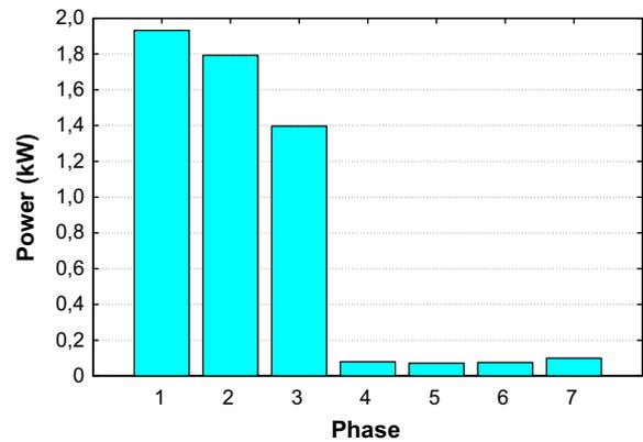
Fig. 1. Example of a load profile  $l_{ahf}$  of a washing machine.
