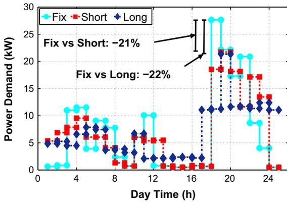
Fig. 6. Peak reduction guaranteed by SA-DSM: aggregate power demand of 20 identical houses (80 homogeneous appliances).
