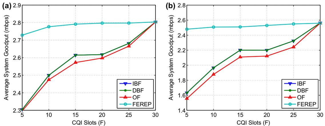
Fig. 4. System goodput for available CQI slots with homogeneous users in (a) pedestrian mobility (b) vehicular mobility.
