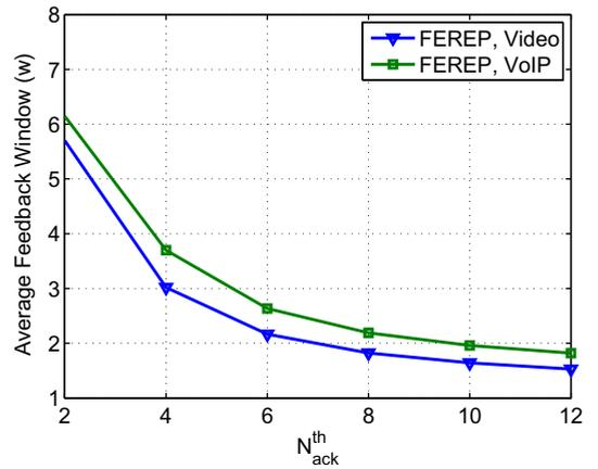
Fig. 6. Average feedback window for different  $N_{ack}^{th}$  values with homogeneous users in vehicular mobility.
