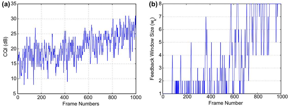
Fig. 5. (a) CQI (b) feedback window for a user with ITU vehicular B channel model.
