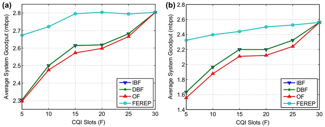
Fig. 7. System goodput for available CQI slots with heterogeneous users in (a) pedestrian mobility (b) vehicular mobility ( $l = 1$ ).
