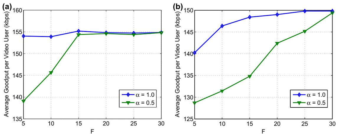
Fig. 9. System goodput for available CQI slots with heterogeneous video users in (a) pedestrian mobility (b) vehicular mobility.
