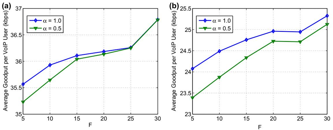
Fig. 8. System goodput for available CQI slots with heterogeneous VoIP users in (a) pedestrian mobility (b) vehicular mobility ( $l = 1$ ).
