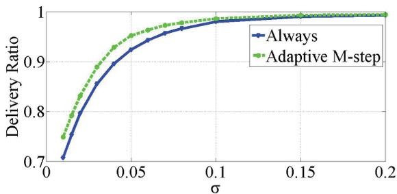
Fig. 3. Comparison of packet delivery ratio with different  $\sigma$  when  $T = 150s$ .
