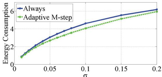
Fig. 4. Comparison of average energy consumption with different  $\sigma$  when  $T = 150s$ .
