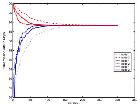
Fig. 7. Rate trajectory under asynchronous subgradient update: non-linear pricing
