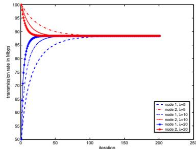
Fig. 6. Rate trajectory under synchronous subgradient update: non-linear pricing
