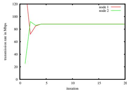
Fig. 4. Rate trajectory under best response: linear pricing
