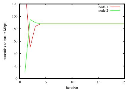
Fig. 5. Rate trajectory under best response: non-linear pricing
