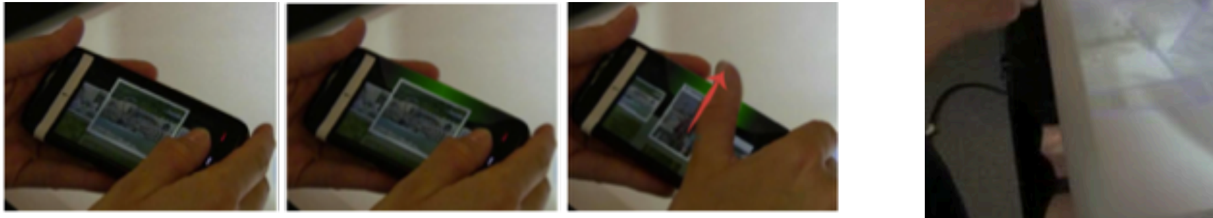
Figure 2— In this example a user is approaching a digital table with their mobile. A halo appears at the edge of the mobile. The user can flick the image towards the halo. When the image slides off the edge of the mobile it disappears and reappears on the table.
