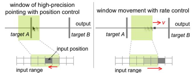
**figure 3.** Mixed control with a movable window
