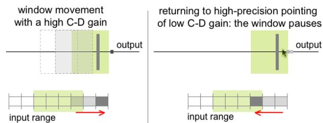
**figure 4.** Position control with a movable window
