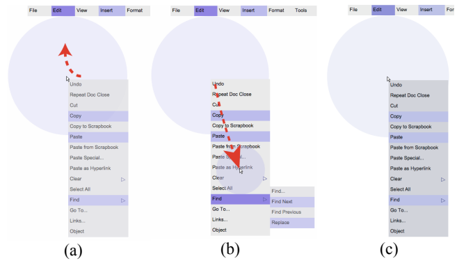
Figure 12. The extended design of bubbling menus. (a) When the user drags the right mouse button, a bubble appears that selects highlighted menu categories. A preview of the corresponding menu follows the cursor as the cursor’s center moves towards the menu bar. (b) The user moves the mouse downwards while dragging. The position of the menu freezes and a second bubble allows for the selection of highlighted items within the menu. (b) Alternatively, the user can release the button to activate the default view of a menu.
