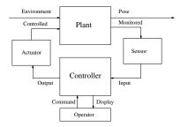
EnvironmentAssumption(environment) AND PlantModel(environment, control, pose, monitor) AND SensorAccuracy(monitor, input) AND ActuatorResponse(output, control) AND ControllerOutput(input, command, output, display) AND OperatorModel(display, command) IMPLIES Requirement(command, environment, pose, display)
