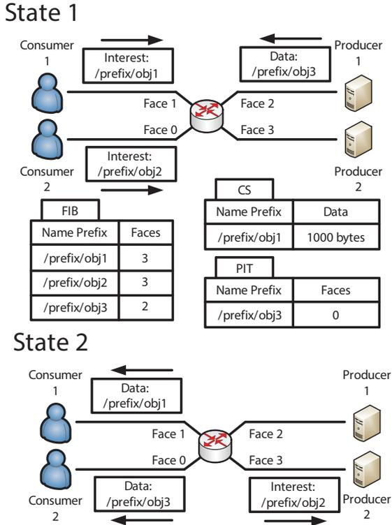
Figure 1. Example illustrating the behavior of a CCN router. Two Interests and one Data packet are received by the router in *State 1*. Given the information contained in the *Pending Interests Table* (PIT), the *Content Store* (CS) and the *Forwarding Information Base* (FIB), in *State 2* the router forwards two Data packets and one Interest.
