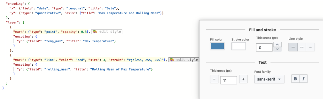
Figure 7.9. Demonstration of the projection for configuring the style of Vega-Lite marks using a form. The Vega-Lite code used in this example is adapted from the Layering Rolling Averages over Raw Values example available on Vega-Lite’s website (0163).
