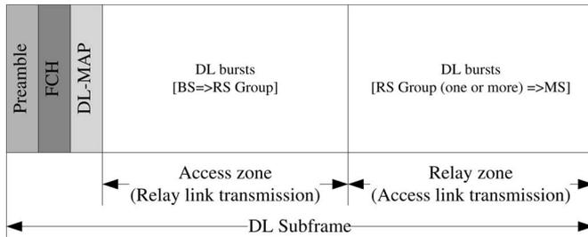
Fig. 2. Modified IEEE 802.16j DL subframe structure for supporting RS grouping.
