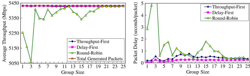
Fig. 10. Performance comparison between different group sizes in terms of (a) throughput and (b) delay without user mobility.
