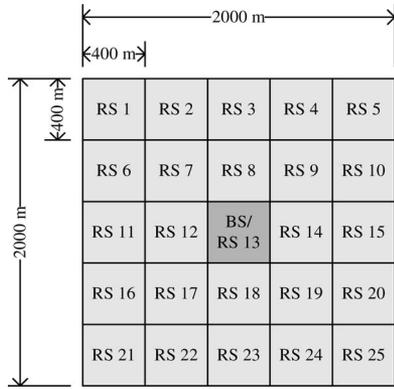
Fig. 6. Simulation topology. Single BS-cell system with a 25-RS-cell grid layout.
