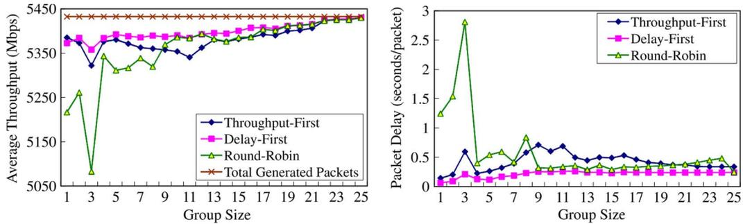
Fig. 11. Performance comparison between different group sizes in terms of (a) throughput and (b) delay with user mobility.
