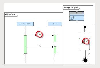
The order of the messages in the scenario's sequence diagram cannot be realized by the state machine order of triggers.
