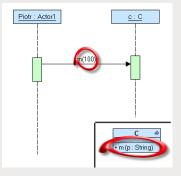
Inconsistency between a type of an argument and a type of a parameter.
