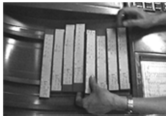
Fig. 1: Stripholders in a stripboard. at the Paris (Athis Mons) en route air traffic control center.
