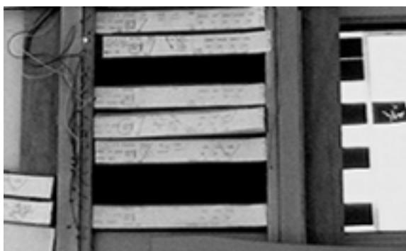
Fig. 2: Stripholders are detected by the electronic stripboard. Writing is captured by the graphics tablet underneath. Information is displayed on the touch screen to the left.
