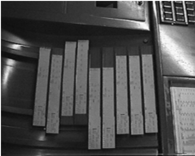
Figure 4 : Flight strips in a strip board at Athis Mons
