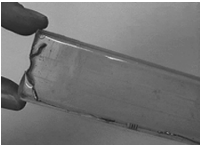
Figure 7: Transparent strip holder with diodes and contacts.
