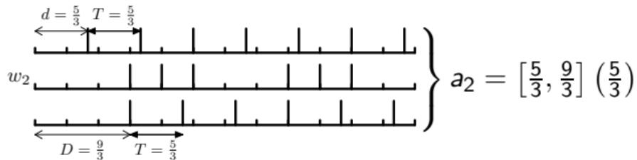
$$\text{concr}([d, D](T)) \stackrel{\text{def}}{\Leftrightarrow} \{w, \forall j \geq 0, T \times j + d \leq [w]_{j+1} \leq T \times j + D\}$$
