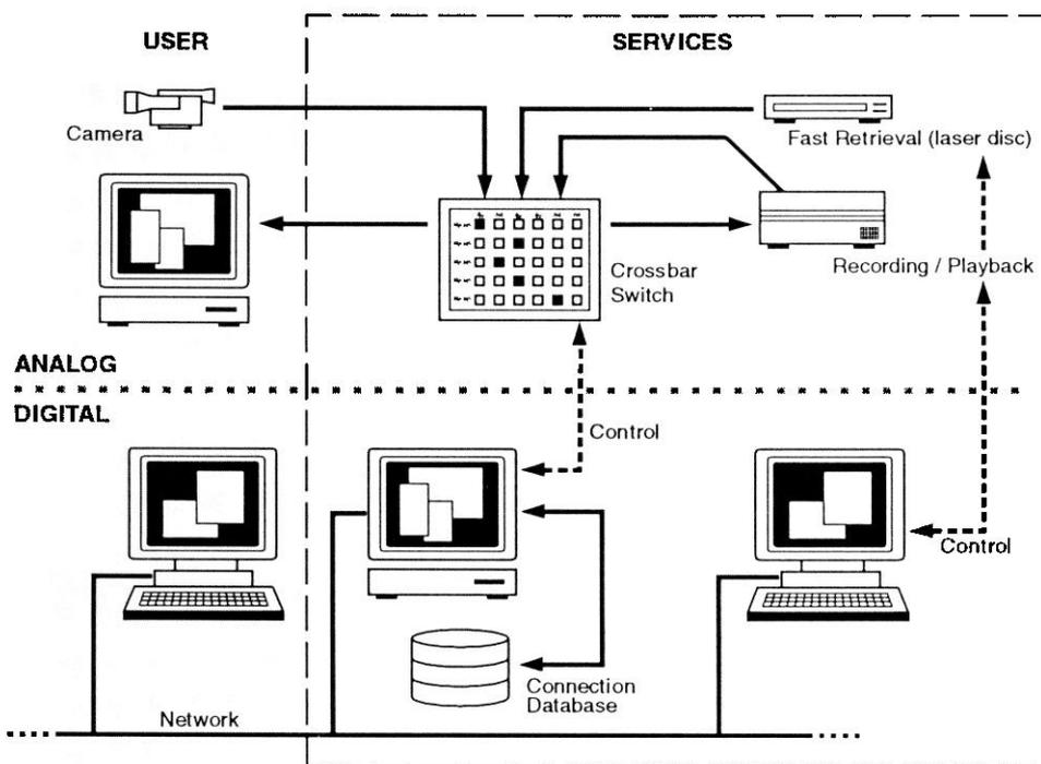
**Figure 4.** From its inception, it was a hybrid analog-digital system. Access control and the state of connection are available from workstations on the network. Additional computers control switching and other services on the analog audio/video network. Note that users may have multiple cameras and monitors. Also, images are sometimes displayed as windows on computer displays.
