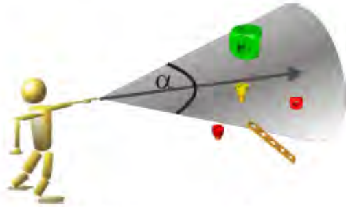
Figure 3.2: One way to model the extension of pointing is using a pointing cone. The cone is a formalized way to account for the decreasing accuracy of pointing when pointing at distant objects.
