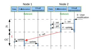
Figure 4: Modification of an object in replicated mode
