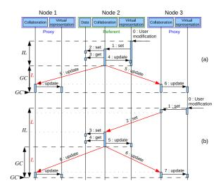
**Figure 3:** Modification of an object in hybrid mode when user is interacting with the referent (a) or with a proxy (b)
