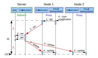
Figure 2: Modification of an object in centralized mode
