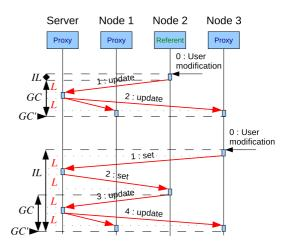
**Figure 5:** Modification of an object in hybrid mode when a client/server architecture is used
