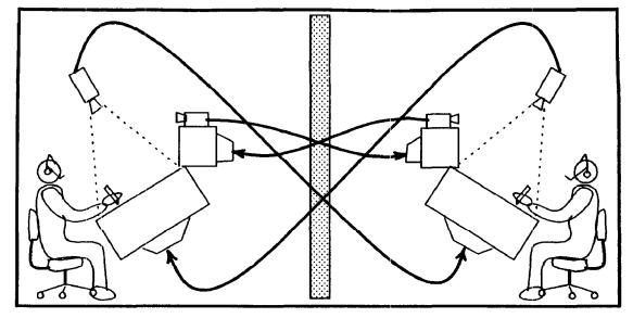
Figure 4: Schematic diagram of VideoDraw connecting remote locations
