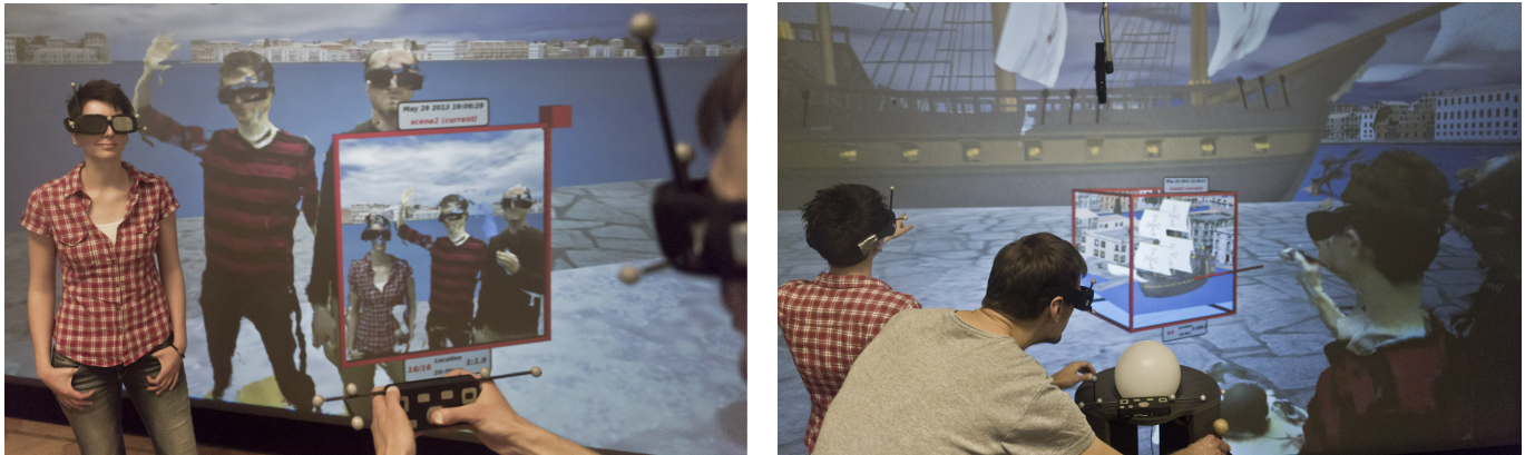
Figure 1. Collaborative interaction with Photoportals. Left: A user takes a virtual photo of a local and two remote collaborators in a virtual city model. Note that the local user (standing on the left) also appears in the virtual photo. Right: Two local users (on the left side) share a box-shaped Photoportal with two remote collaborators (on the right side). A remote user operates a virtual pointer inside the portal to manipulate the ship model in the background at a convenient scale and distance while the other users provide guidance from their individual viewpoints.
