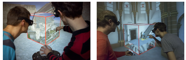
Figure 7. Using Photoportals as a WIM. The image on the right side illustrates the benefits of implicit geometry clipping for wayfinding inside a virtual building. Note the 3D video avatars of remote users in the miniature view.
