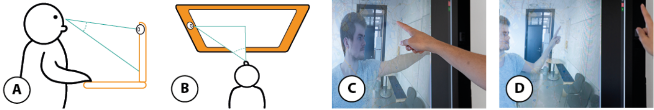
Figure 7: The problem of parallax. A-B: Horizontal and vertical parallax. C-D: Perceiving one's body in real space during gesture vs. perceiving one's own body representation in the camera feedback.
