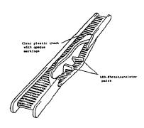
Figure 3: Cutaway view of an Allison Research Slider
