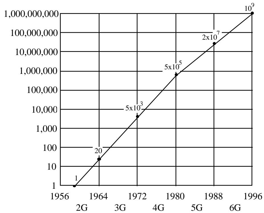
**Figure 1 The number of devices on a chip**
