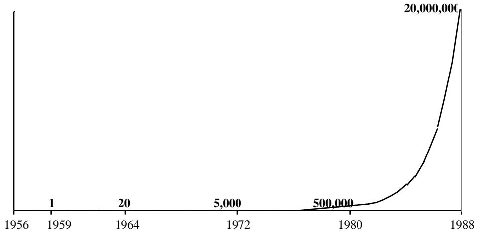
**Figure 2 The number of devices on a chip on a linear scale**
