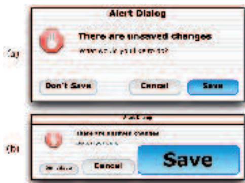
Figure 2: With Semantic Pointing, objects can have a visual size different from their size in motor space, i.e. they can "feel" smaller (or larger) than they look. This is achieved by dynamically controlling the mapping between mouse movements and cursor movements. Here it is applied to a dialog box: (a) visual appearance, (b) motor space. The default button is made bigger in motor space and therefore easier to select, while non-interactive elements such as labels or dangerous ones such as the Don't Save button are made smaller in motor space and therefore harder to select.
