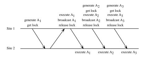
**Figure 5.6** The DistView toolkit uses a token-based locking scheme to help improve response time for typical usage patterns. Site 1 needs to acquire a token from a remote site for the first operation  $A_1$ . For subsequent operations that require the same lock, no token needs to be acquired over the network, leading to good response times
