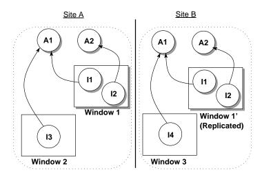
**Figure 5.11** The state of the multi-user application at sites A and B after the user at site B imports Window 1 in the DistView-based application. Appropriate objects necessary for sharing windows efficiently are replicated and maintained consistent on subsequent updates
