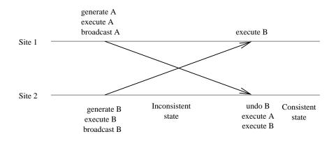
**Figure 5.7** The use of undo/redo strategy for optimistic concurrency control. At site 2, execution order is made consistent with that at site 1 by undoing execution of B and then executing A and B. Site 2 is temporarily in an inconsistent state with respect to site 1
