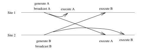
**Figure 5.5** The use of ordered broadcast protocols to achieve data consistency. Delivery and execution of message B must be delayed at site 2 so that delivery/execution order is consistent with that at site 1. Also, B is executed in a different state than when it was generated, possibly leading to an unintended document state
