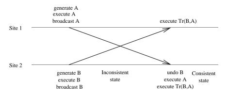
**Figure 5.9** The use of transformations to achieve data consistency and consistency with users' intentions in an optimistic manner using undo/redo. In this case, all sites execute operations in the same sequence, if necessary after reordering operations
