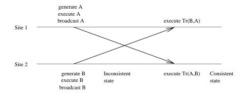
**Figure 5.8** The use of transformations to achieve data consistency and consistency with users' intentions in an optimistic manner, without the use of undo/redo. Sites may do operations in different order and transformations must satisfy constraints that ensure consistency
