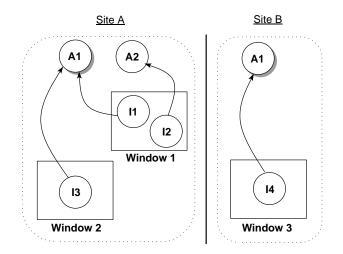
**Figure 5.10** The state of a multi-user application at sites A and B before sharing of Window 1 in a DistView-based application. A1 and A2 are application objects, and I1, I2, I3, and I4 are interface objects
