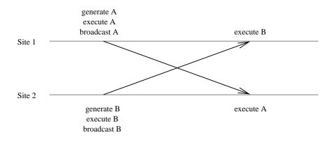
**Figure 5.4** A scenario of the document state becoming inconsistent at different sites. Without concurrency control, the two operations A and B are executed in different orders at different sites, possibly leading to different states
