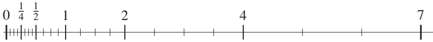
Figure 2.2. The positive floating-point numbers in the toy system \beta = 2, p = 3, e_{\min} = -2, e_{\max} = 2 .
