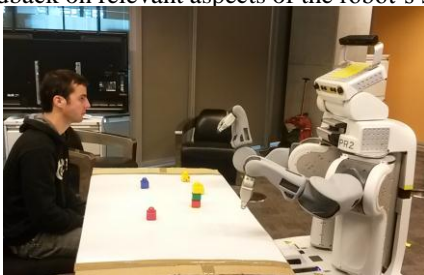
Fig 1: Example of joint action where some objects are out of reach. The human has to understand when the robot is unable to reach the objects.
