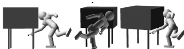
(b) Behaviour of the 39-DOF Humanoid: Reaching goal under Balance and Collision constraints
